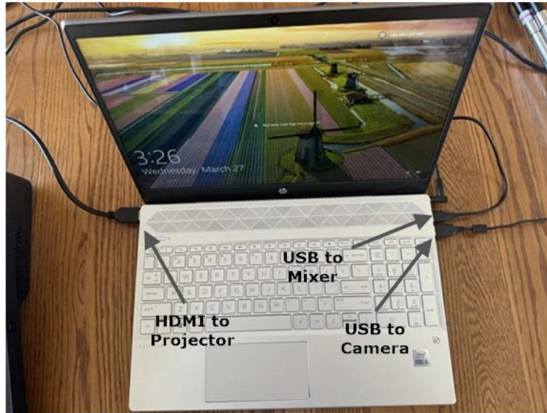
Figure 4. Laptop Connections (typical)
